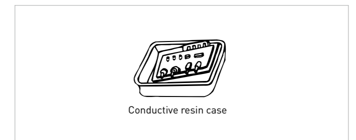
Fig. 3 A battery-mounted PC board was inadvertently brought into contact with a conductive resin case. The battery charge was exhausted.
